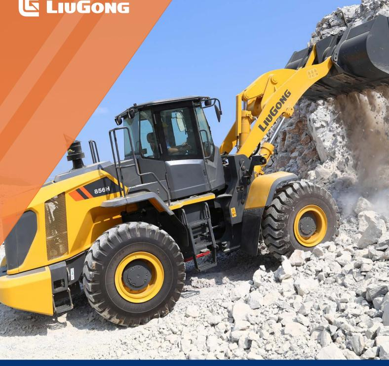
Engine 162 kW (217 hp / 220 ps) @ 2,200 rpm **Gross Power** 149 kW (200 hp / 202 ps) @ 2,200 rpm **Net Power Operating Weight Standard Bucket Size Standard Breakout Force Standard Dump Clearance**
